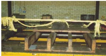
TTI have designed and made splices in Kevlar ropes up to 1000 tonne nominal break load and polyester ropes up to 1500 tonnes break load. The Kevlar strand splice was developed using special techniques to ensure strands were tensioned and tucks made at constant pitch.
