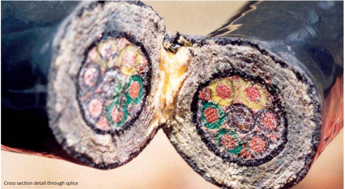
Cross section detail through splice
